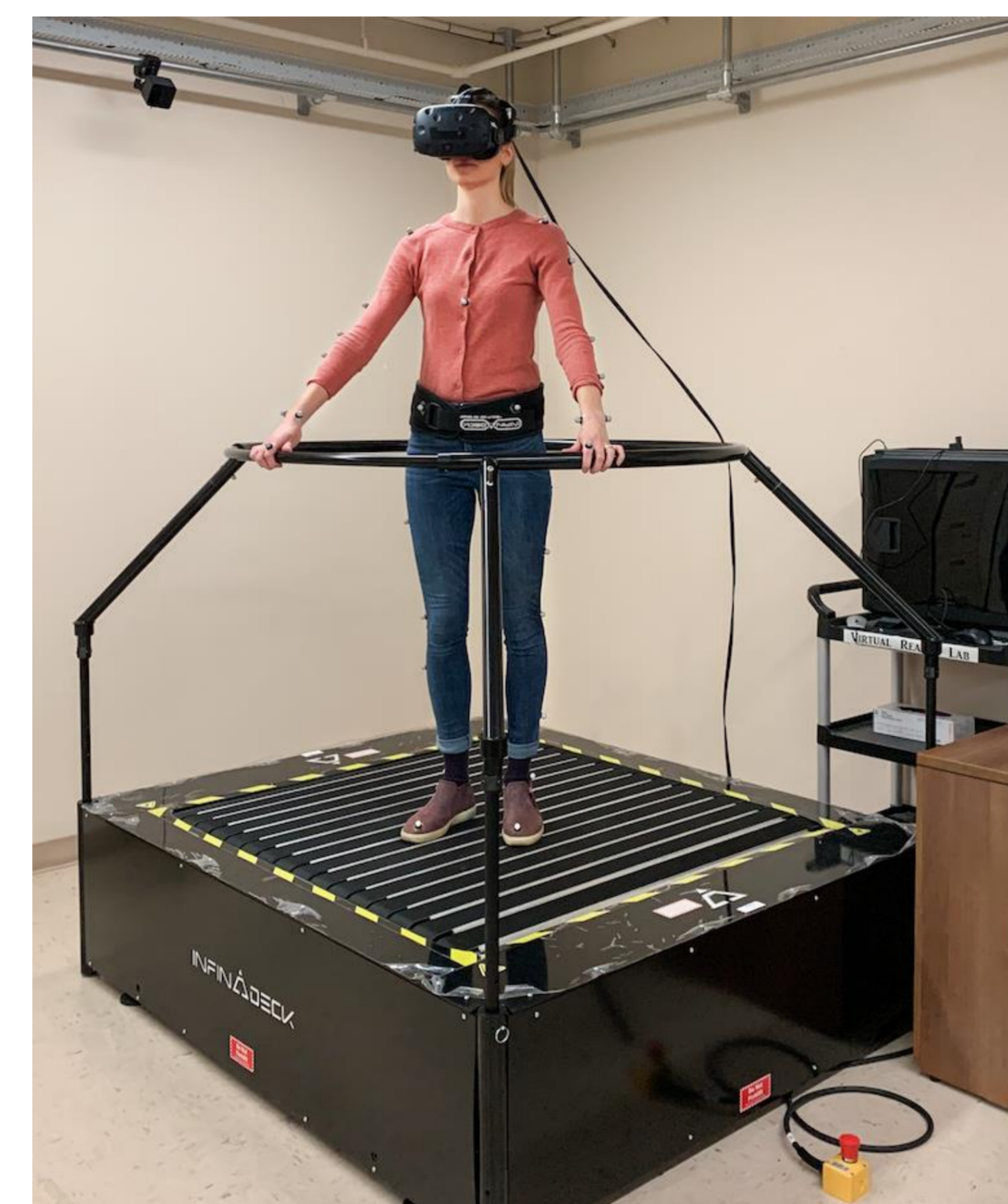
Fig 2. OMT treadmill set up with reflective markers positioned according to the Plug-in Gait model.
